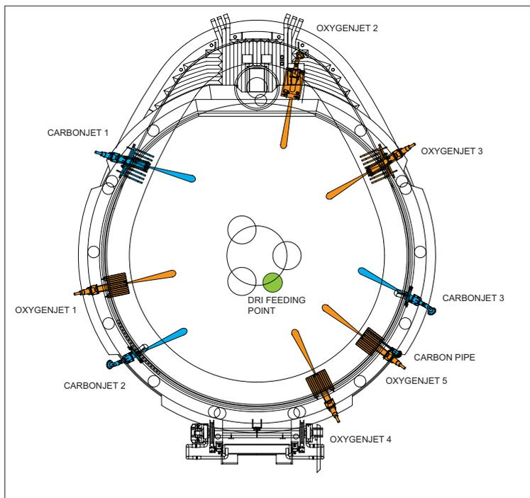
Fig 2 Oxygen and carbon injector layout
