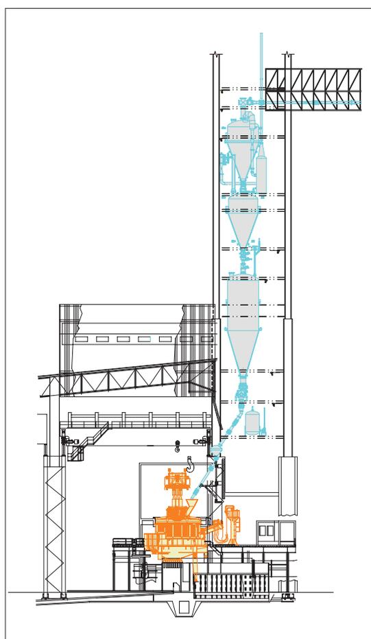
Fig 1 EAF and HYTEMP DRI tower
