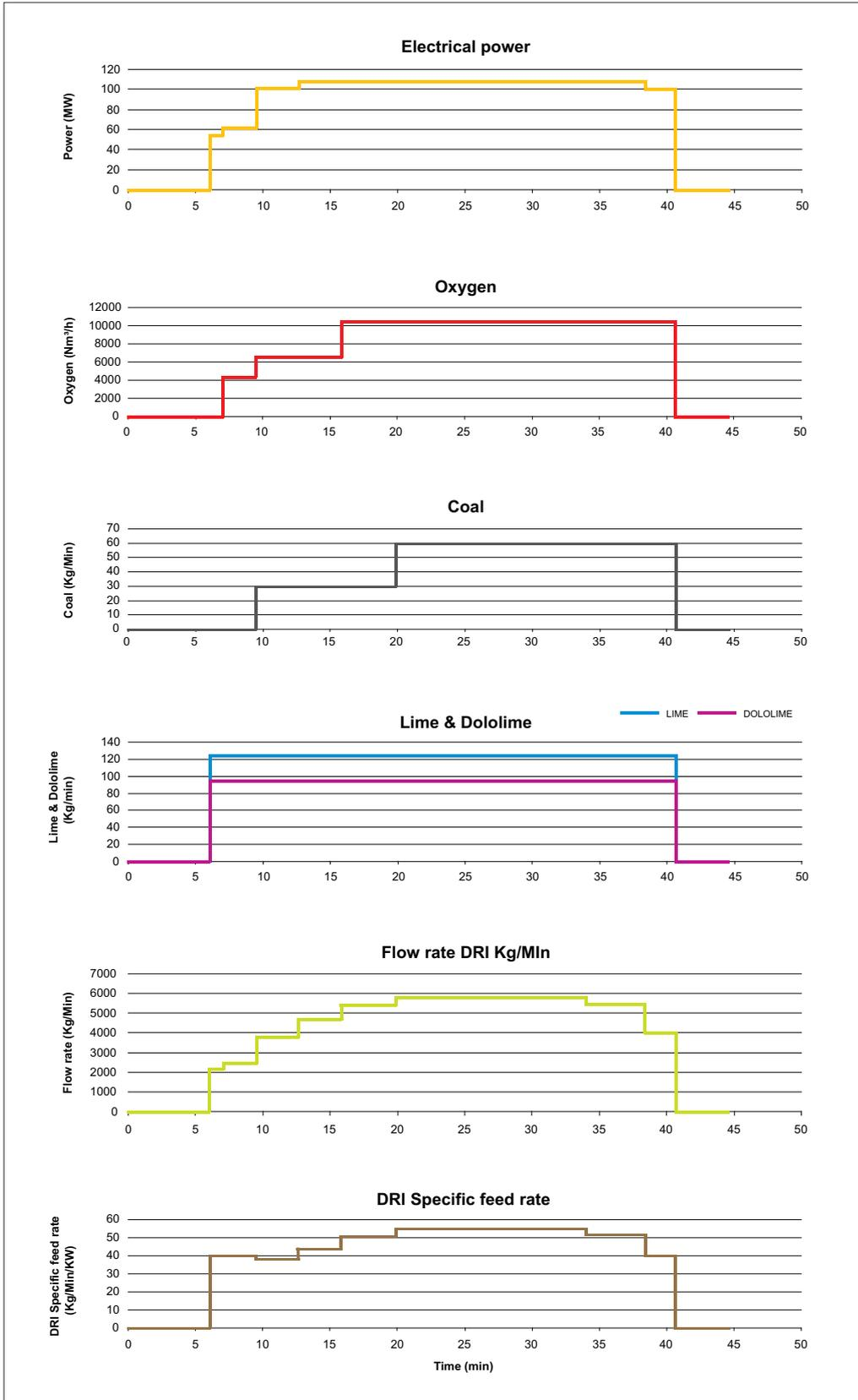
Fig 3 Melting profiles
