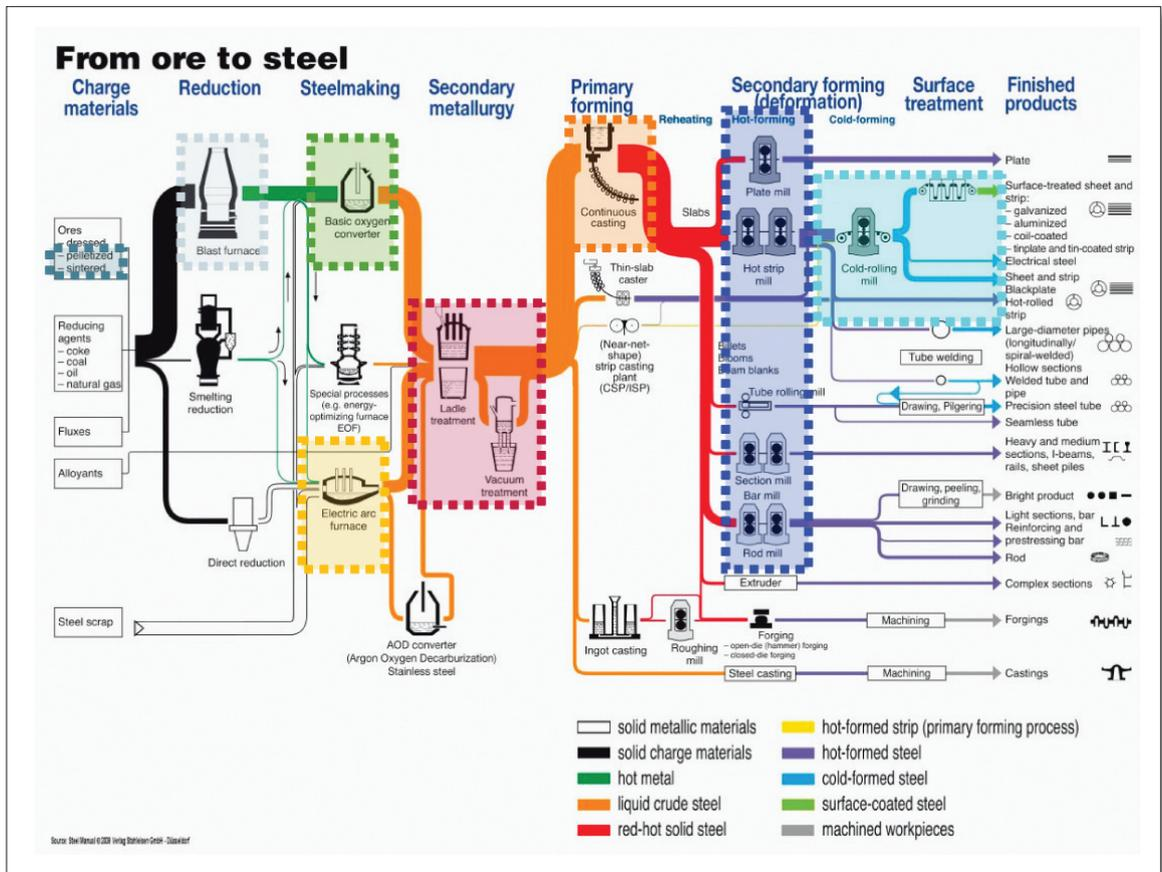
Fig 1 From ore to steel – the processes
