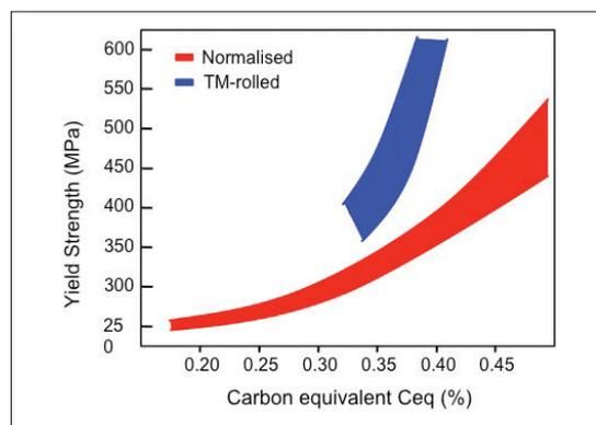
Fig 2 Relationship between yield strength and carbon equivalent
