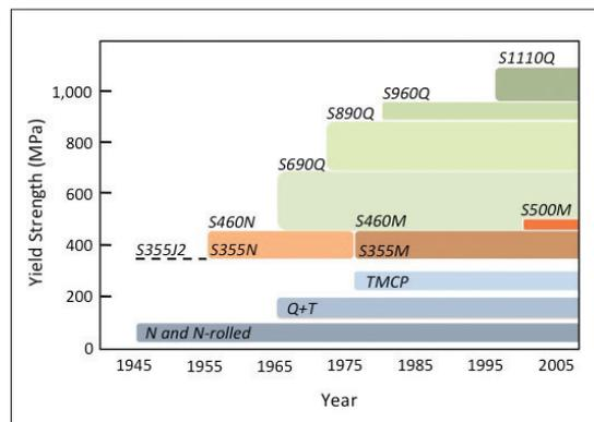
Fig 1 General evolution of structural steel
