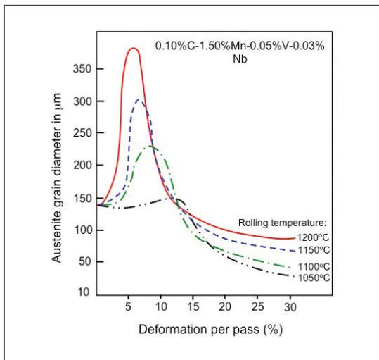
Fig 4 Recrystallised austenite grain size in pre-rolling of microalloyed steels
