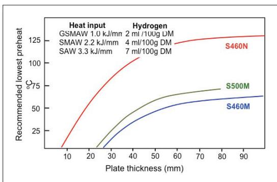
Fig 5 Calculated preheat temperatures as a function of plate thickness – moderate restraint
