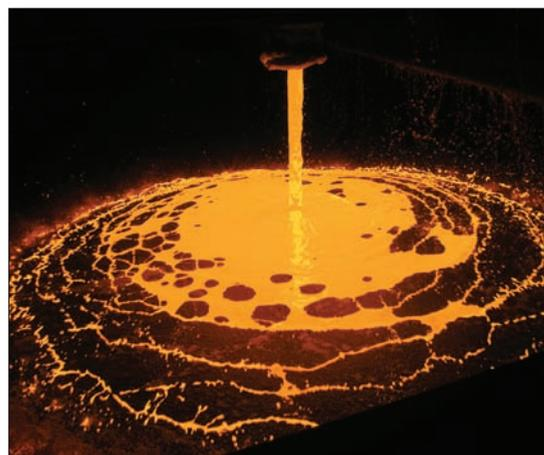
Fig 3 Granshot granulation on spray-head – typical metal umbrella formation
