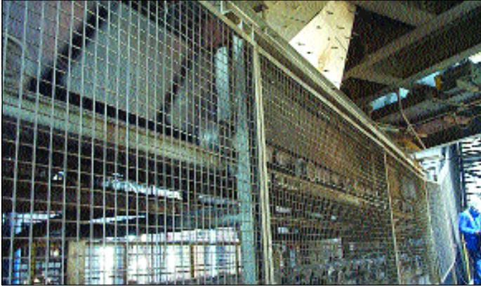
● **Figure 5** Charging point for hot material with heat insulated hood and Inertisation
