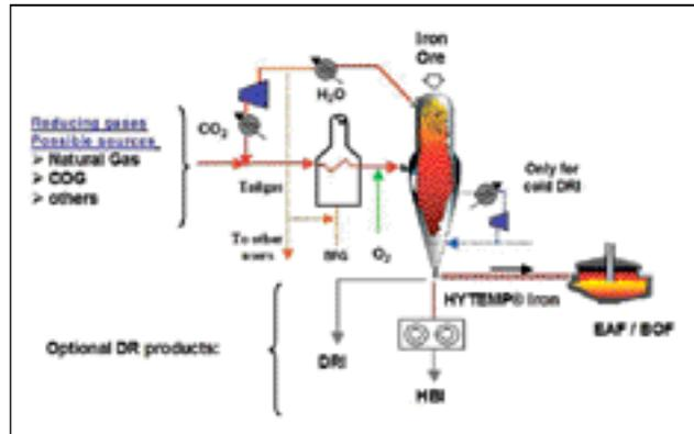
● **Figure 4 Principles of HYL III – process schematic**
