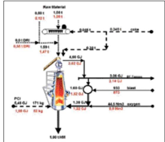
● **Figure 7** Example of charging DRI to blast furnace
