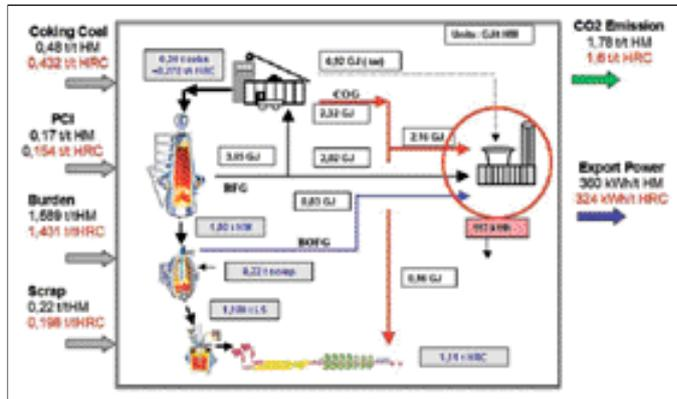
● **Figure 1 Overall balance for integrated steel works based on HRC production**
