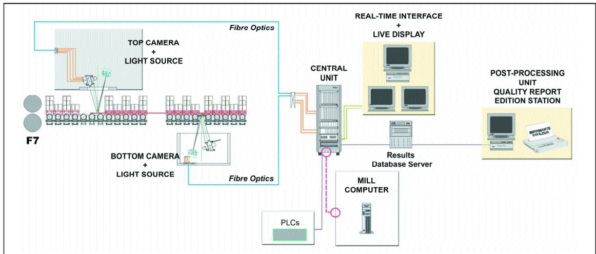
● **Figure 2 Arcelor Dunkerque HSM: Location of equipment and global system architecture**
