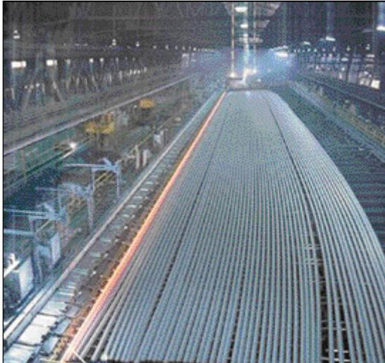
● **Figure 2** Walking beam 120m cooling bed
