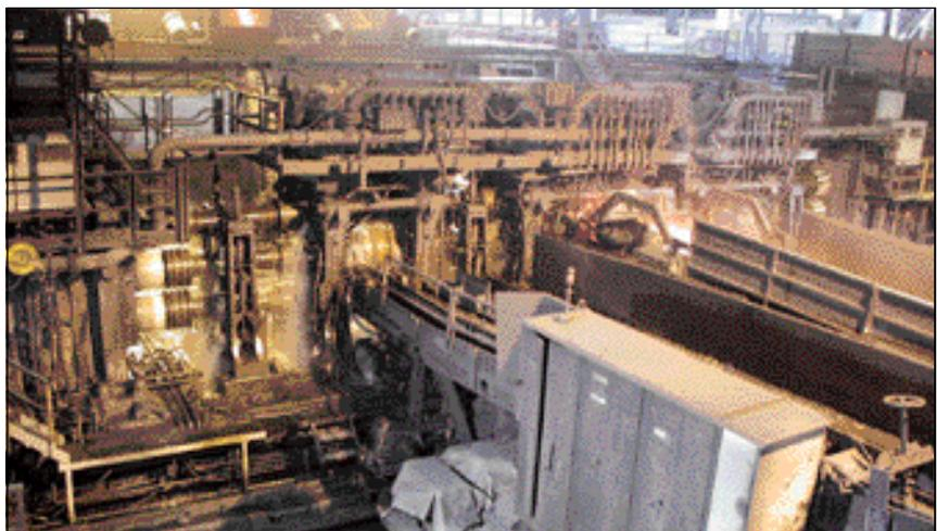
● **Figure 4** Existing finishing mill with two 3-high and one 2-high stands
