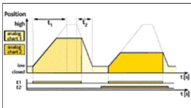
● **Figure 7** Capacity and lambda adjustment by analogue and digital signals
