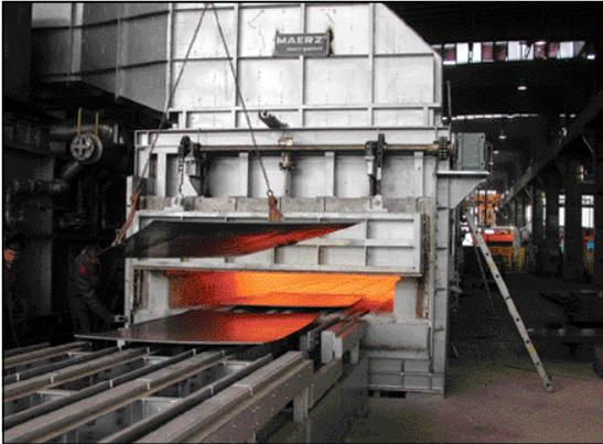
● **Figure 2** Lifting hearth furnace sheet charge line
