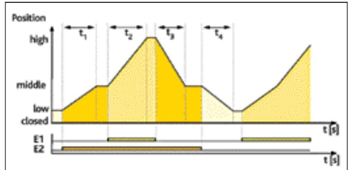
● **Figure 6 Control example: IC 40 actuator – two-stage operation**
