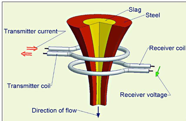
● **Figure 3 Basic measurement principle of electromagnetic slag detection**
