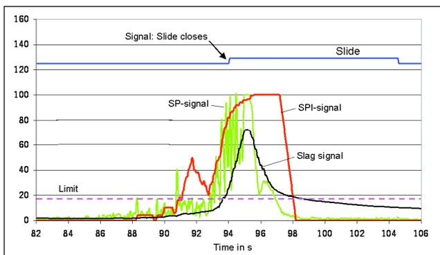
● **Figure 4 Slag detection signal profiles**
