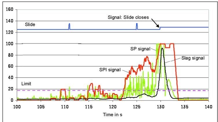
● **Figure 5** Slag detection during slag particle carry over
