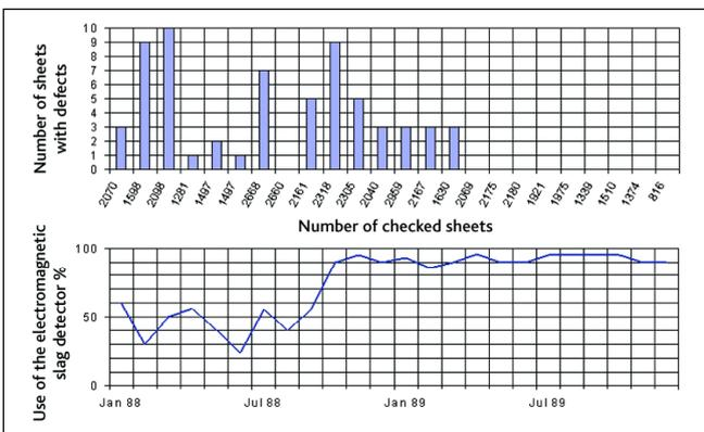
● **Figure 1** Improvement of cleanliness for tinplate coils by electromagnetic detection
