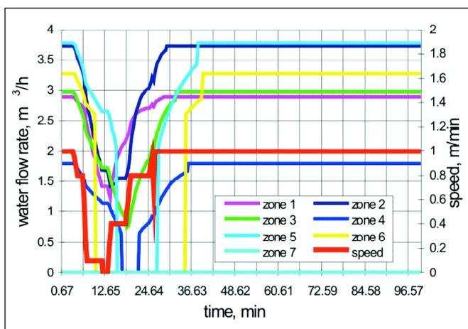
● **Figure 2** Water flow changes by zone, depending on casting speed
