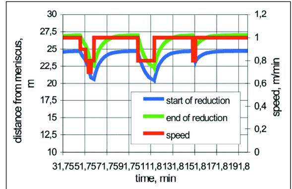
● **Figure 4 Location of soft reduction zone limits depending on casting speed**
