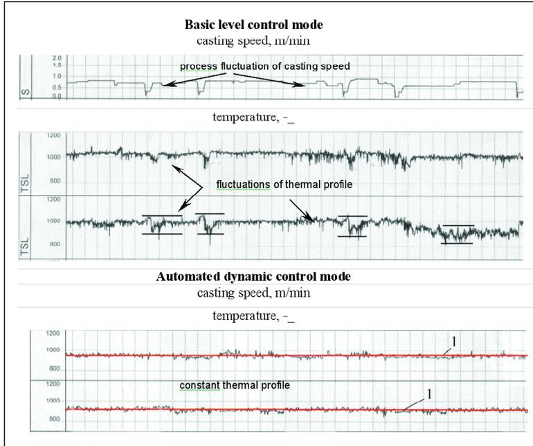
● **Figure 3 Comparison of water flow rates controlled from basic (blue) and automated levels (red) at CCM No.3, Magnitogorsk Steel Works**
