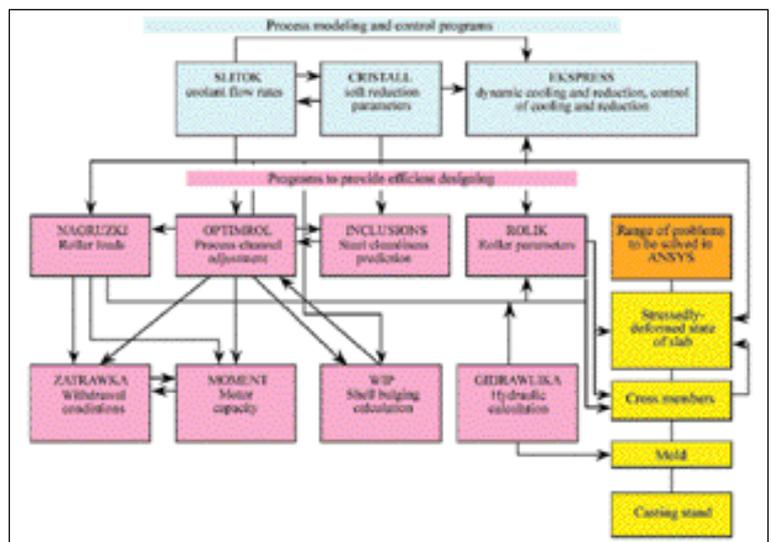
● Figure 1 MNLZ calculation package. Software communications diagram
