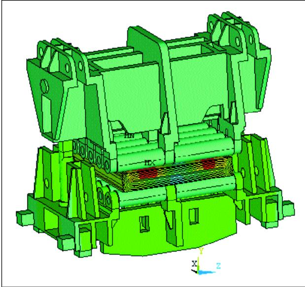
● **Figure 6** Spectrum of movements for the soft reduction unit strand system
