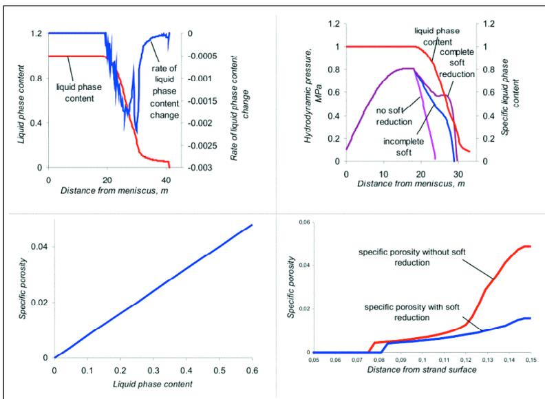
● **Figure 5 Results of calculation modelling for strand solidification with and without soft reduction**
