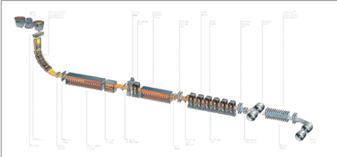
● **Figure 8** EFS flat steel mini-mill layout, Egypt
