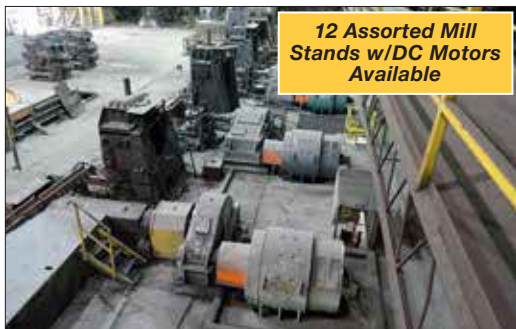
(4) Neumann 16" x 27 1/2" Vertical & Horizontal (2) High Mill Stands w/600 HP Dc Motors
