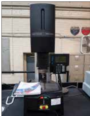
Wilson Rockwell 2001R Digital Hardness Tester
