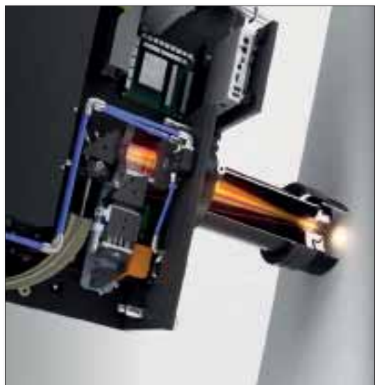
Fig 1 Schematic of the LIBS process, showing a pulsed laser beam (in red) generating a plasma on the surface and an associated spectral of light being collected for analysis.
