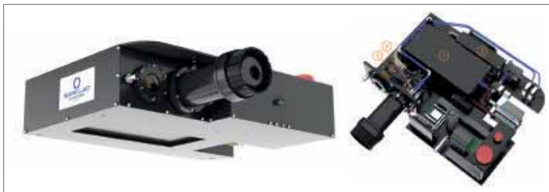
Fig 2 LIBS demonstration unit with (1) the laser, (2) the laser controller, (3) the laser beam focusing unit and (4) the light collecting unit
