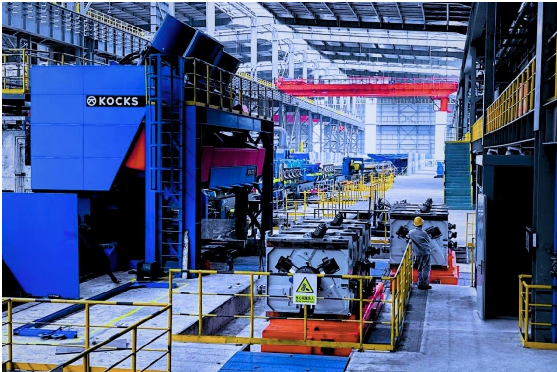
Image Caption: First bar on KOCKS' largest Reducing & Sizing Block RSB® 500++/4
