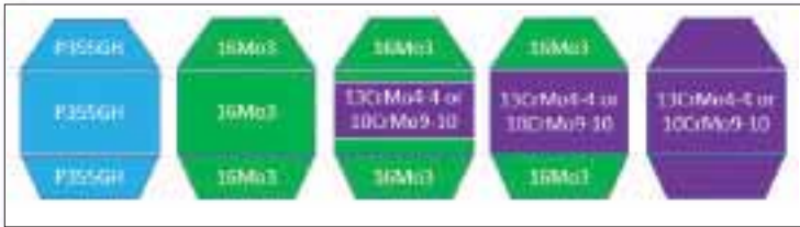
Fig 2 Steel grade combinations in a vessel shell (temperature resistance and life increasing L to R)
