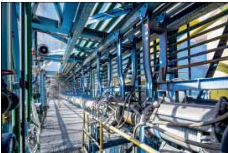
🕒 Fig 7 Zerobucket® Hytemp pneumatic transport of DRI
