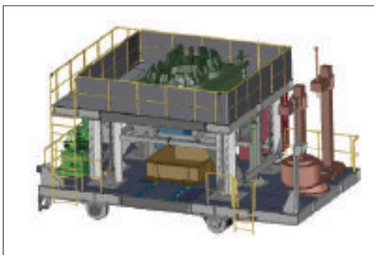
⌚ Fig 16 Service car with scraper and gunning robot (picture from SMS group)
