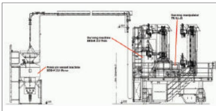
⌚ Fig 20 Automatic gunning installation, on snorkel service car, connected by hose swing
