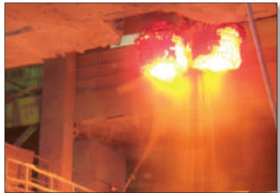
Ⓐ Fig 14 High material loss with manual gunning
