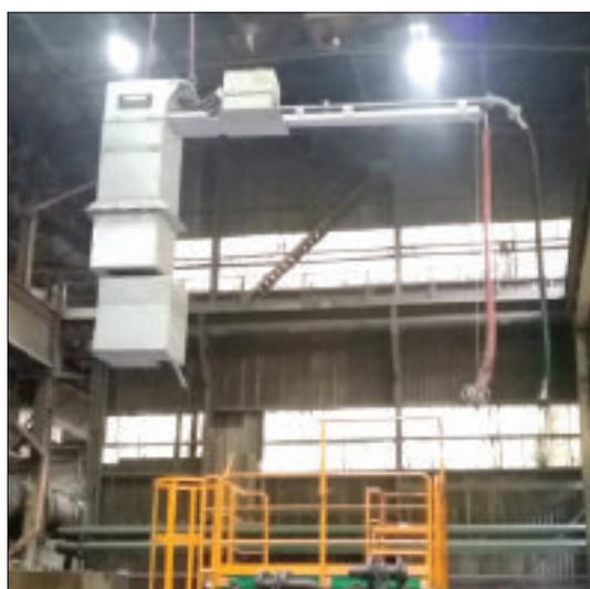
Fig 11 PNEUTOP robot moved by a crane
