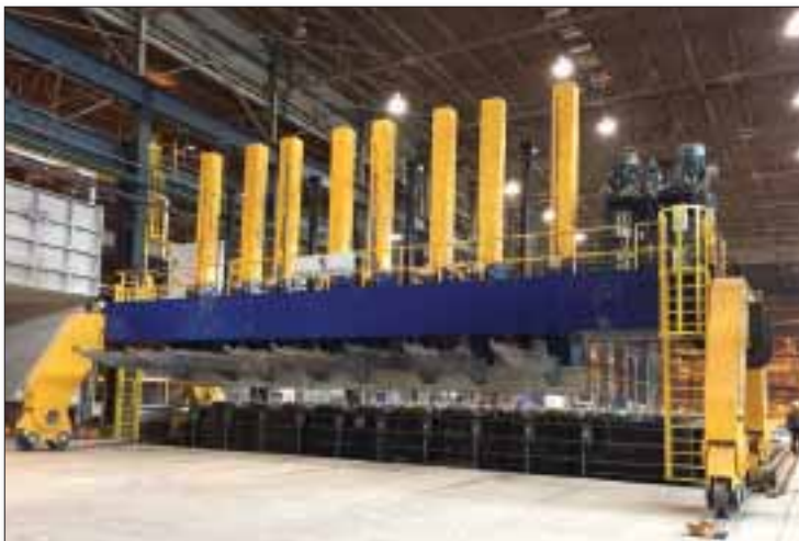
Fig 5 A fully automatic fork transfer system for the heat treatment of crankshafts with a load capacity of 75t
