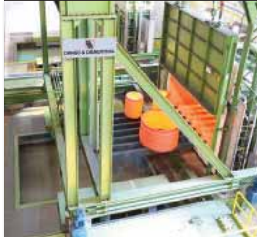
ⓐ Fig 2 An automatic handling system for a quenching facility that is adapted to transfer
