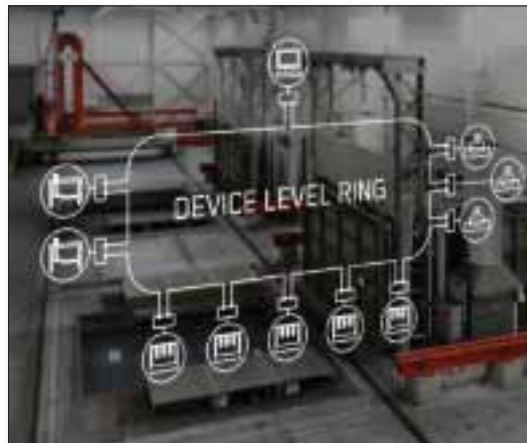
ⓐ Fig 3 The Device Level Ring connects the individual machines within a network
