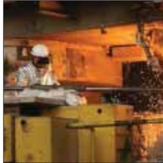
Fig 3 Operator lancing the taphole
