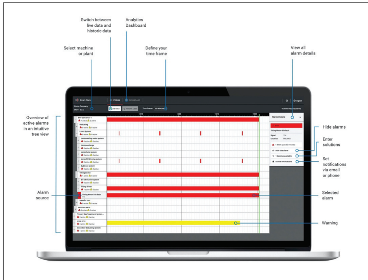
Fig 4 Smart Alarm visualises all the relevant alarms on a dashboard
