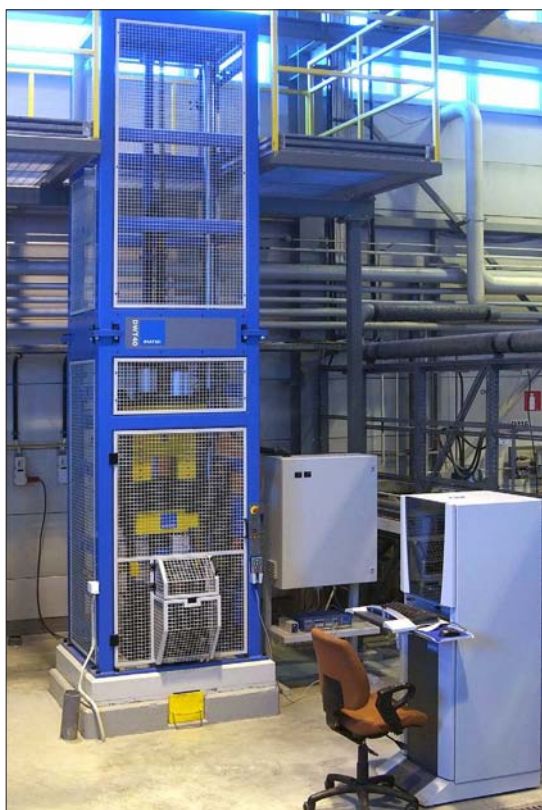
© Fig 2 Imatek DWTT with 25,000J capacity
