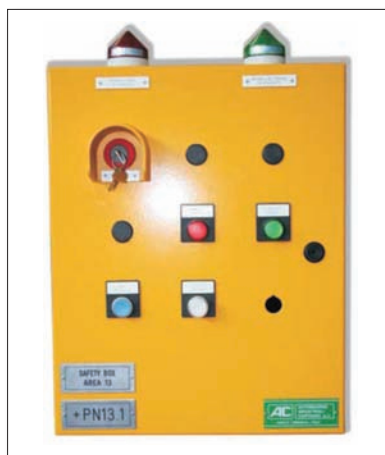
Fig 6 Typical safety box
