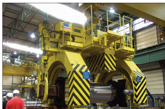
Fig 2 Special tongs for rolls with chock tilter equipment
