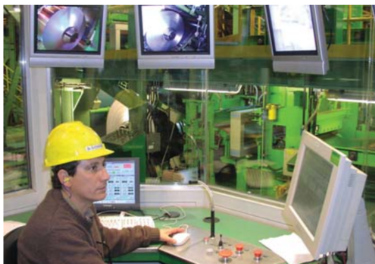
Fig.3 Highly automated recoiling line in Ternium (Siderar- Techint group), Argentina
