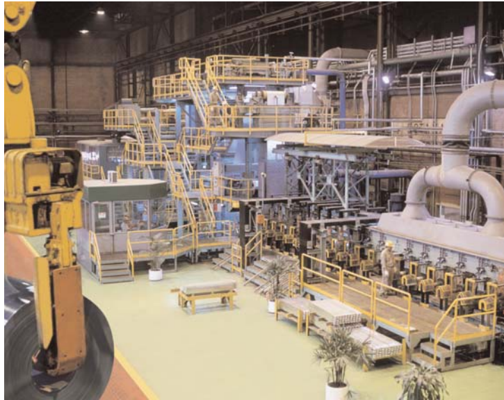
Fig.4 Electrolytic tinning line in Ternium (Siderar- Techint group), Argentina
