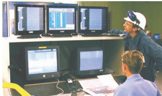
Fig.6 Automotive galvanising line surface inspection pulpit
