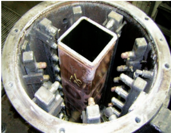
Fig.6 Water-spray mould without top flanges
