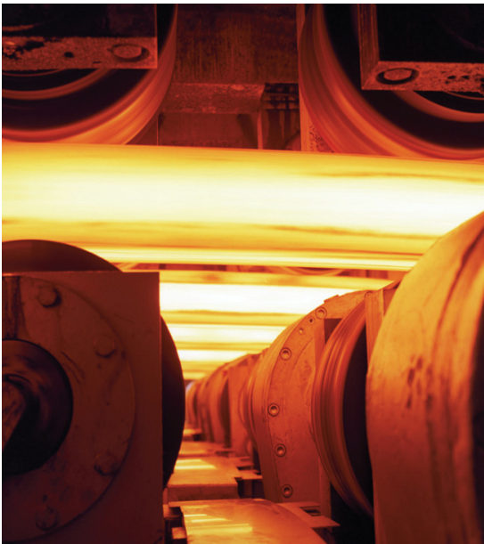
Fig.2 Billets during soft reduction
