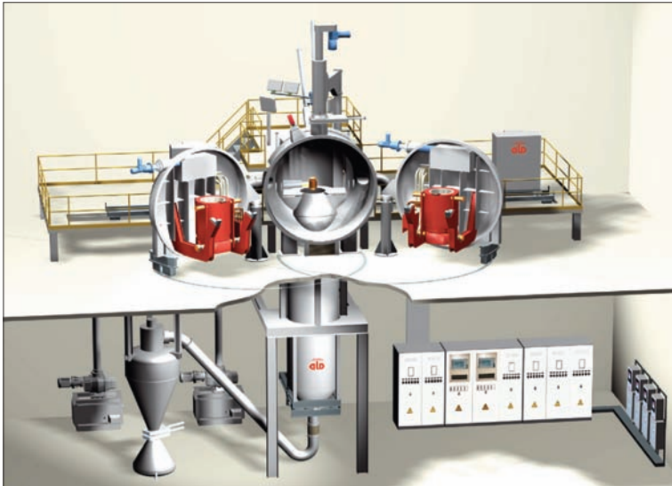
Fig.5 Schematic of a large VIGA plant with a charge weight of 2 x 2t [2]
