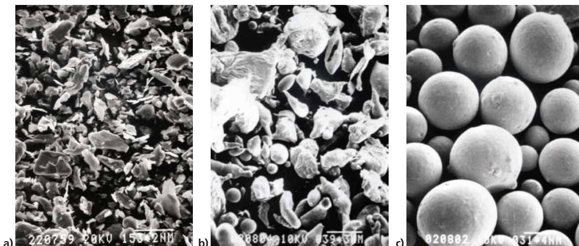
Fig.1 Typical powder shapes, a) - milling , b) - water atomisation, c) - inert gas atomisation
