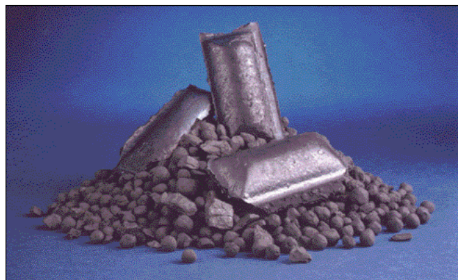
● Figure 5 Direct Reduced Iron (DRI) and Hot Briquetted Iron (HBI)
