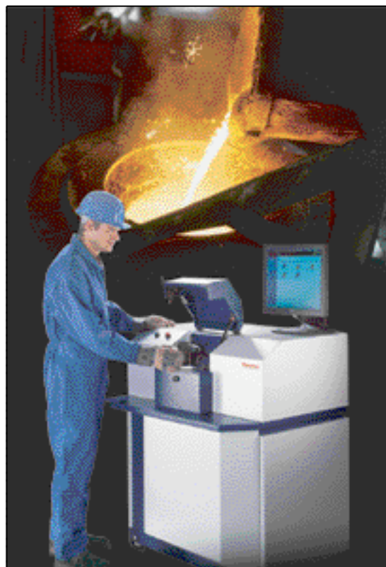
● Figure 1 The ARL QUANTRIS CCD-based metals analyser
