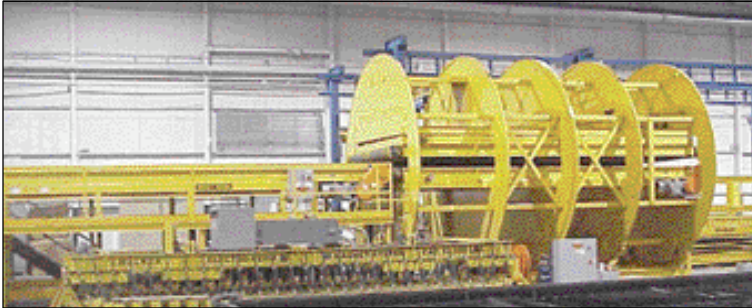
● Figure 2 Inlet table and barrel inverter. Inverter turns 3.6t plate over for de-slugging
