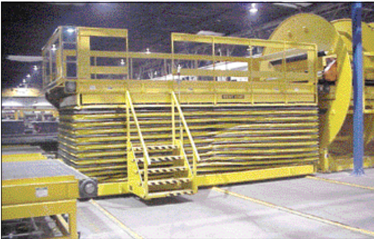
● Figure 3 Outlet table (left) aligns with barrel inverter prior to receiving transferred plate
