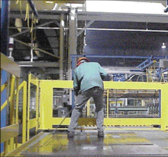
● Figure 4 Slag removal with chipping tool
