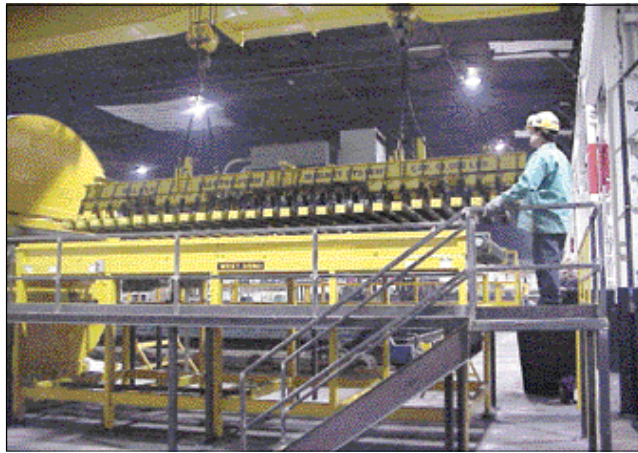
● Figure 1 Overhead crane with magnet carrying burned plate above inlet table. The table has a steel mesh conveyor on it
