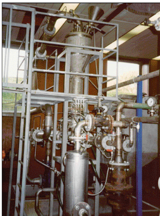
● Figure 2 Dissolution section of the laboratory pilot plant
