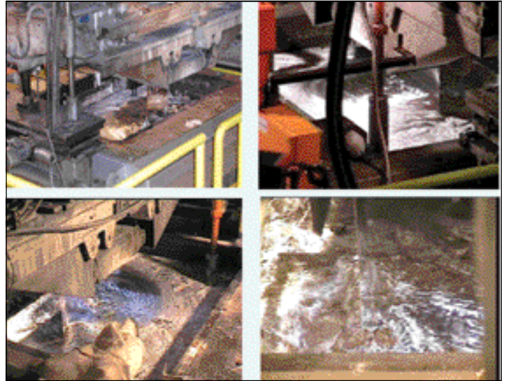
● Figure 8 Hot-dip galvanising with CVGL
