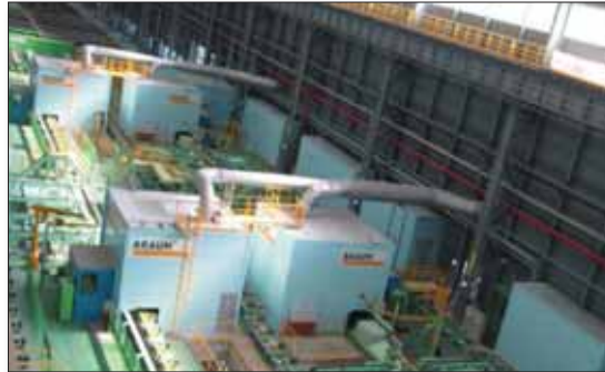
Fig 16 Four HP grinding machines at HYUNDAI Steel, Dangjing, Korea (grinding machines with material handling system in grinding area)
