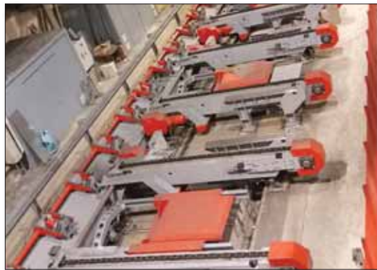
Fig 17 HP grinding machine at VOESTALPINE Stahl, Leoben-Donawitz, Austria (with material handling equipment at loading area)
