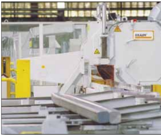
Fig 15 HP abrasive cut-off machine for cutting-off defective billet ends
