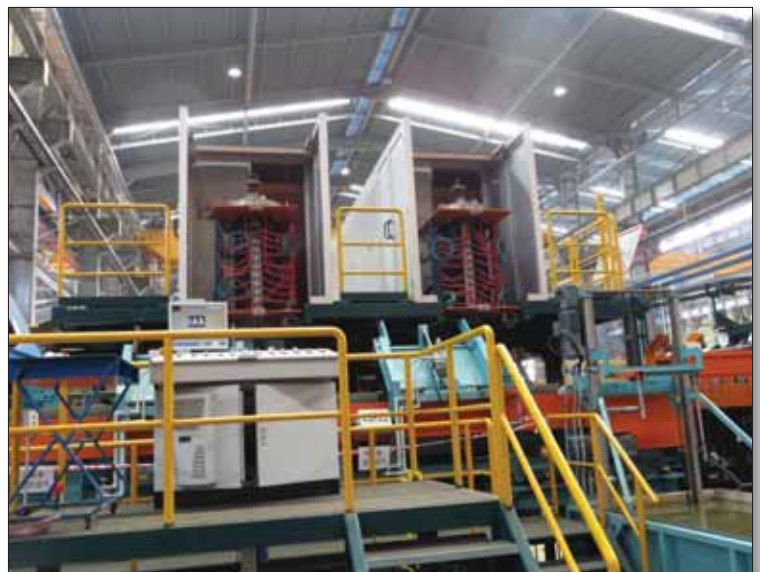
Ⓐ Fig 6 Example of multi-zone heating
