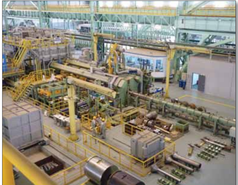
ⓐ Fig 7 60 MN extrusion press, Baosteel Group, China, tube O.D. 48-323mm
