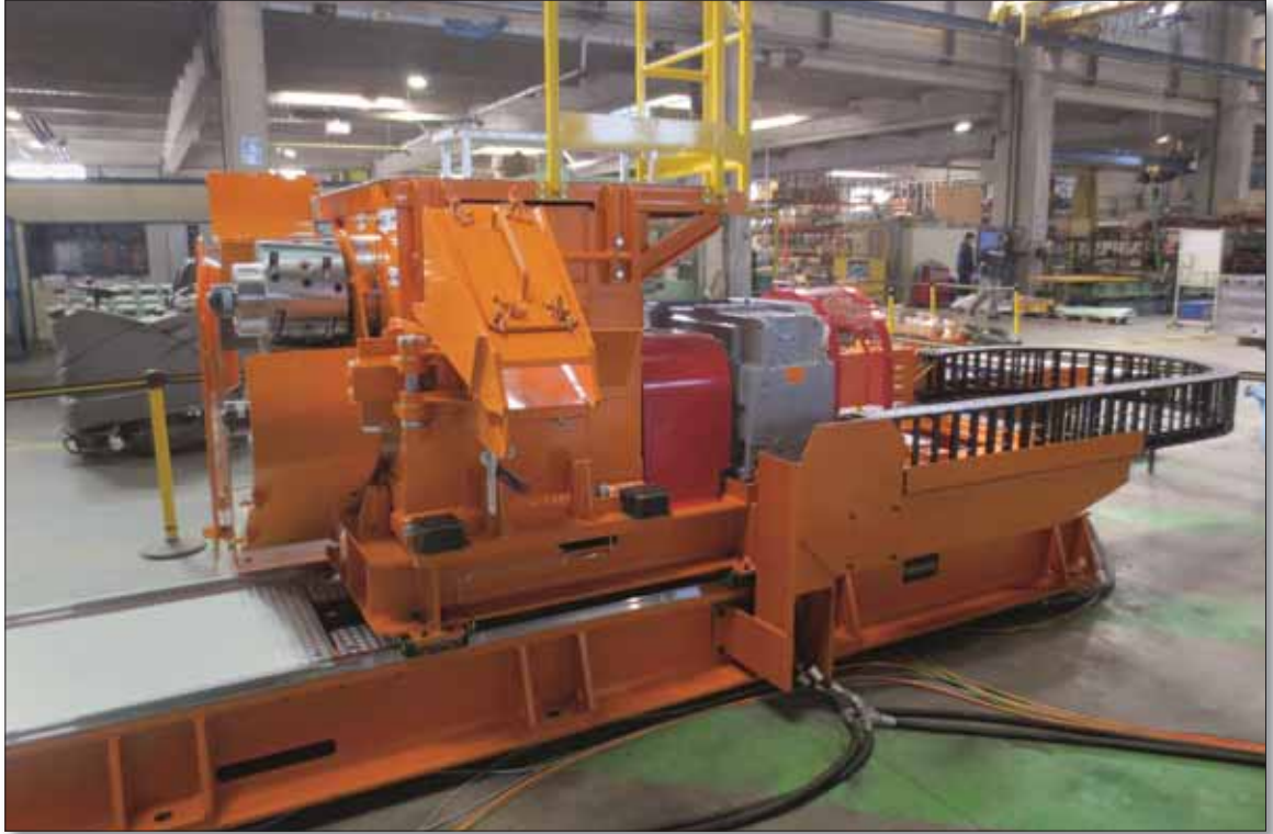
Ⓐ Fig 2b Side trimmer workshop testing
