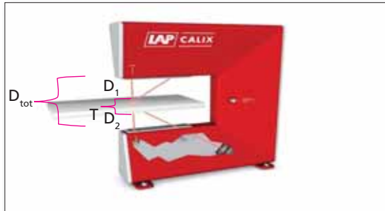
Ⓐ Fig 5 Laser-based thickness gauge
