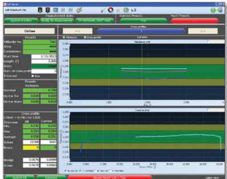
Fig 7 Typical online display of a traversing laser thickness gauge including cross profile
