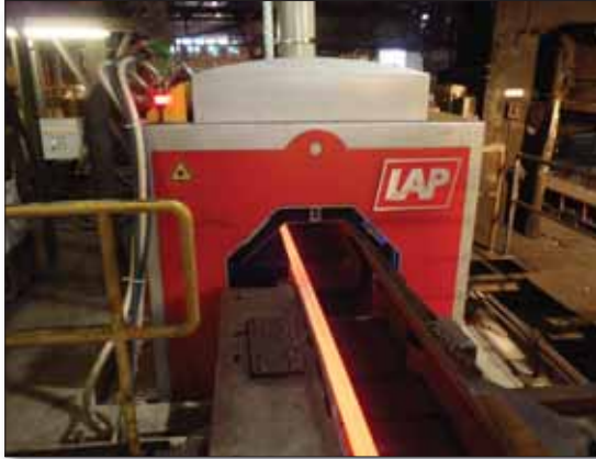
ⓐ Fig 2 Contour gauge in the production line
