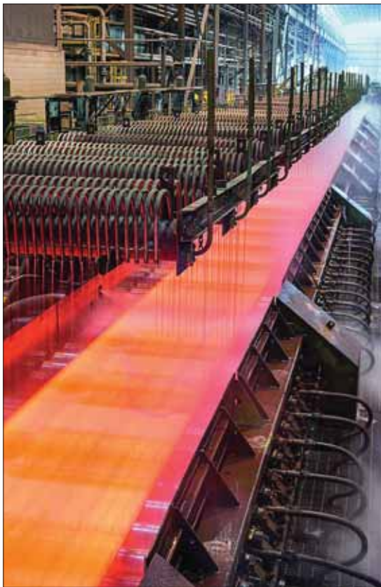
Fig 3 Run out table cooling
