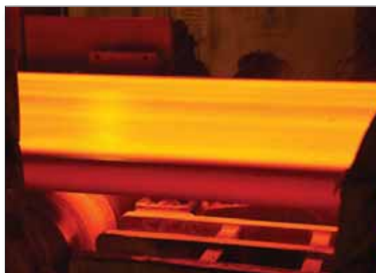
Fig 5 Thin slab at caster exit
