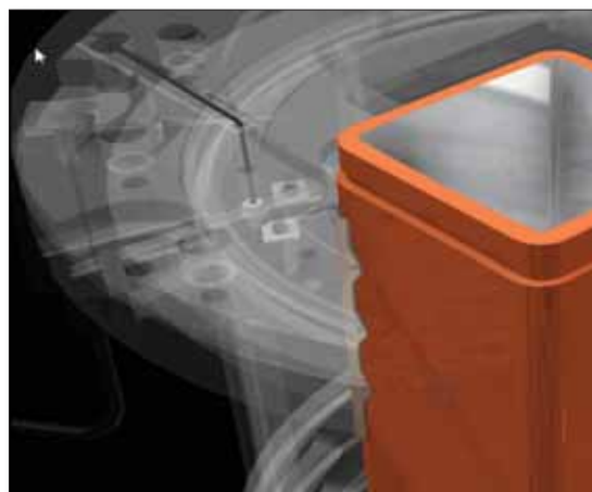
Fig 2 Scheme of sensor array mounted on a mould tube with cabling from wet side to dry side
