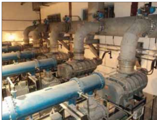
Ⓐ Fig 11 Arrangement of parallel vacuum modules in the pump room of Mechel VOD-plant in Russia (from ref 4)
