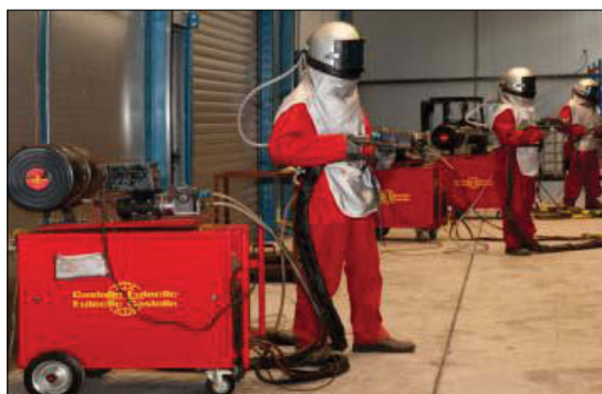
Fig 4 Arc wire spraying equipment
