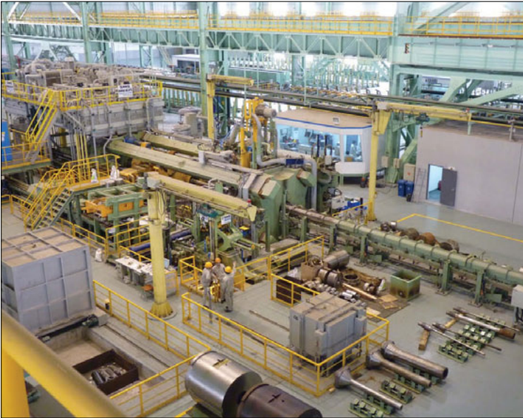
Fig 7 60 MN extrusion press, Baosteel Group, China, tube O.D. 48-323mm
