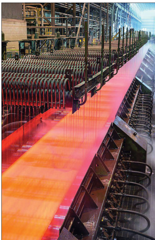
Fig 3 Run out table cooling
