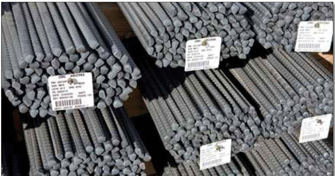
Ⓐ Fig 1 Bundled rebar
