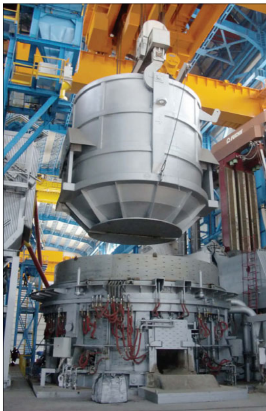
Fig 3 165t Telescopic EAF and large single bucket charge operating in the Middle East
