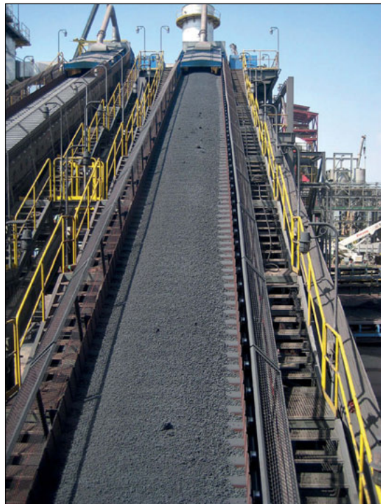
Fig 1 AUMUND conveyor type KZB for handling hot pellets
