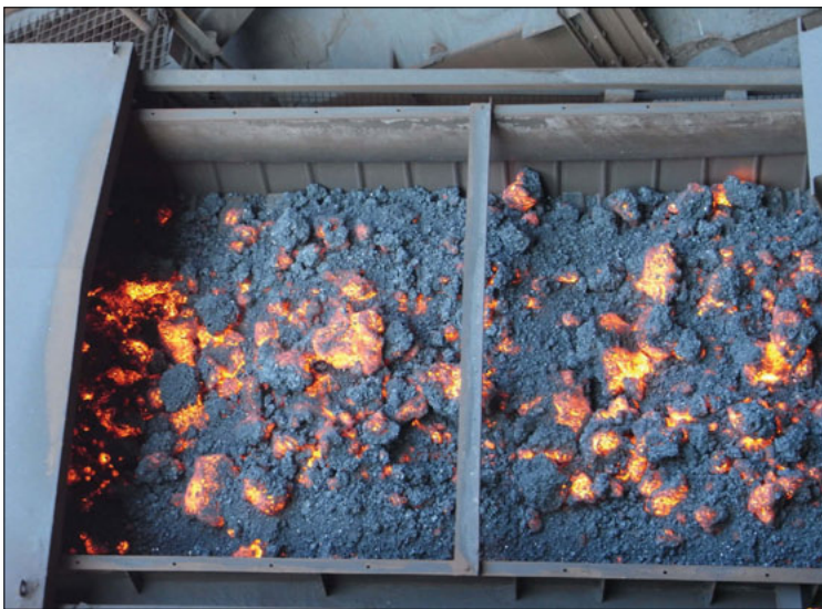
Fig 3 Conveyor type KZB-S transporting hot sinter
