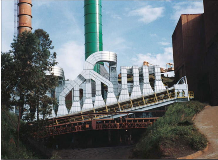
Fig 2 AUMUND conveyor type KZB-KP for cooling hot pellets
