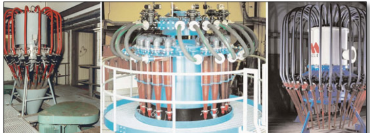
Fig 2 Examples of hydro-cyclones
