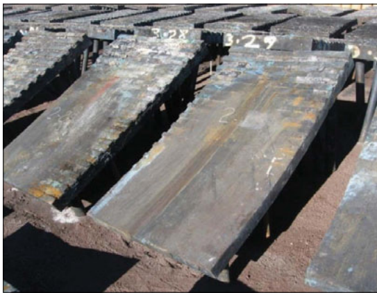
Ⓐ Fig 8 Wear caused by abrasion
