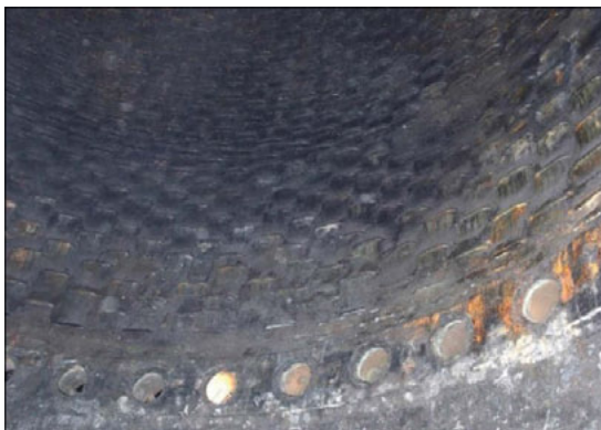
Ⓐ Fig 9 Plate-cooled Bosh
